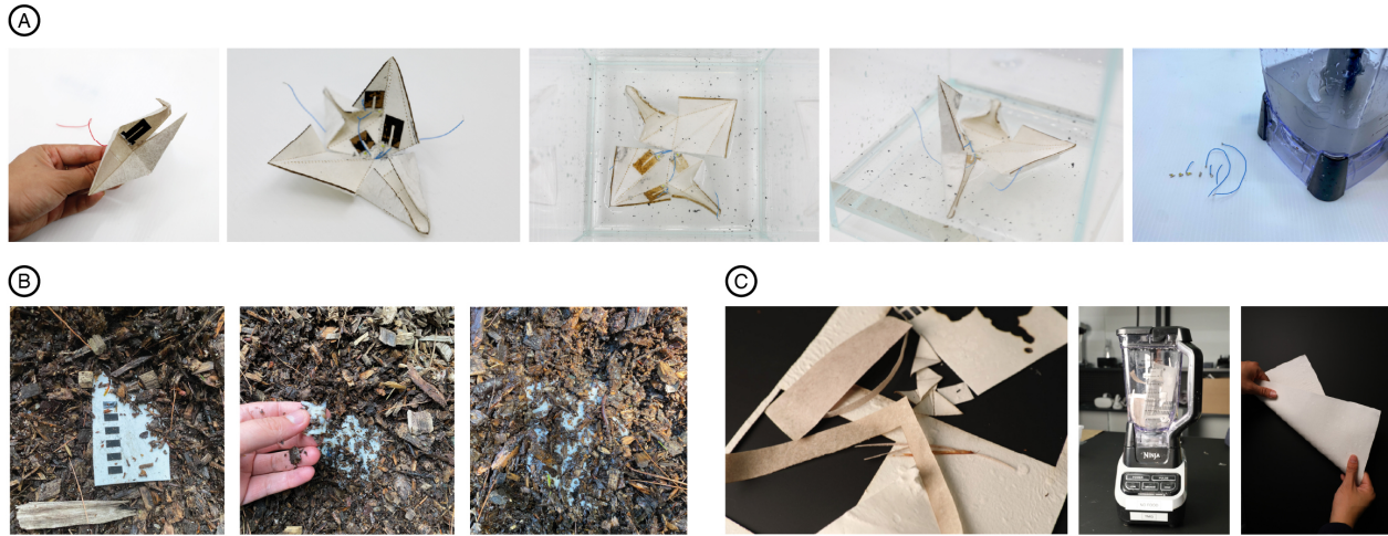
Figure 16: BioLIG sensors and circuits can be recycled and disposed of in different ways. (A) leverages the water-soluble properties to separate conventional electronics from the substrate. (B) sensors can also be composted with no harm to the soil. (C) material cut-offs and scraps created during the subtractive manufacturing process can be blended to make new substrates.
