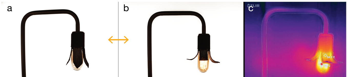
Figure 9: In this application, we demonstrate the aesthetic affordances of 'livingness' with a blooming lamp. When one turns on the light, the heat warms the fibers causing them to contract and lift the petals.
