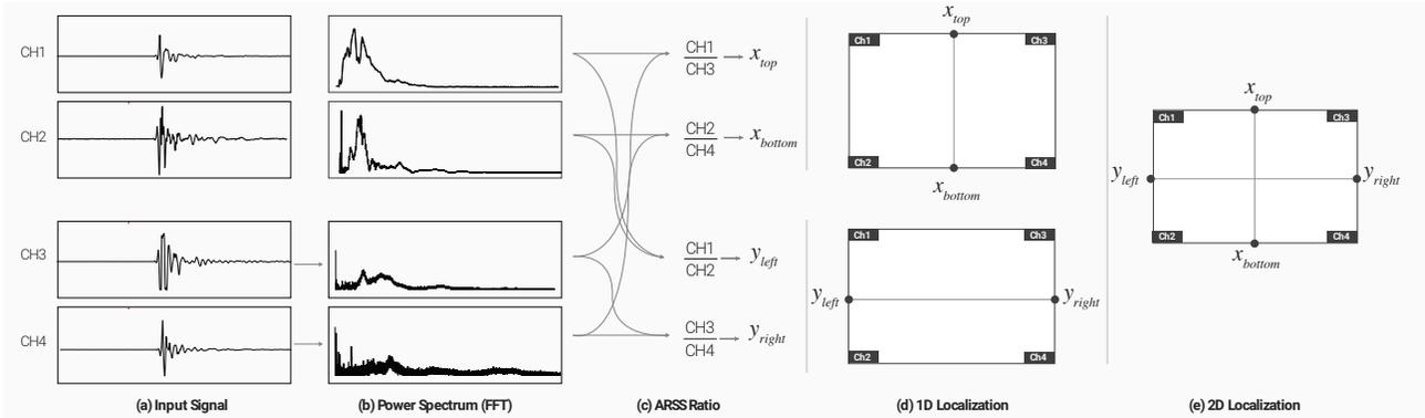
Figure 7. Adaptive Received Signal Strength (ARSS) localization technique. We calculate the  $x$  and  $y$  coordinates of the contact point by taking the ratio of power between channel-pairs on each edge of the sheet. Our localization point is the intersection of the vertical line between  $x_{top}$  and  $x_{bottom}$ , and the horizontal line between  $y_{left}$ ,  $y_{right}$ .
