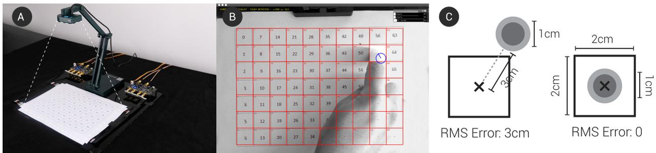
Figure 8. The procedure of technical evaluation. (a) VibroAware setup with printed 20cm x 14cm sheet printed with seventy 2cm x 2cm cells aligned with an overhead camera. (b) Evaluation software displaying the view from camera and alignment between printed test sheet and software grid. (c) Criteria for measuring touch accuracy for each cell.
