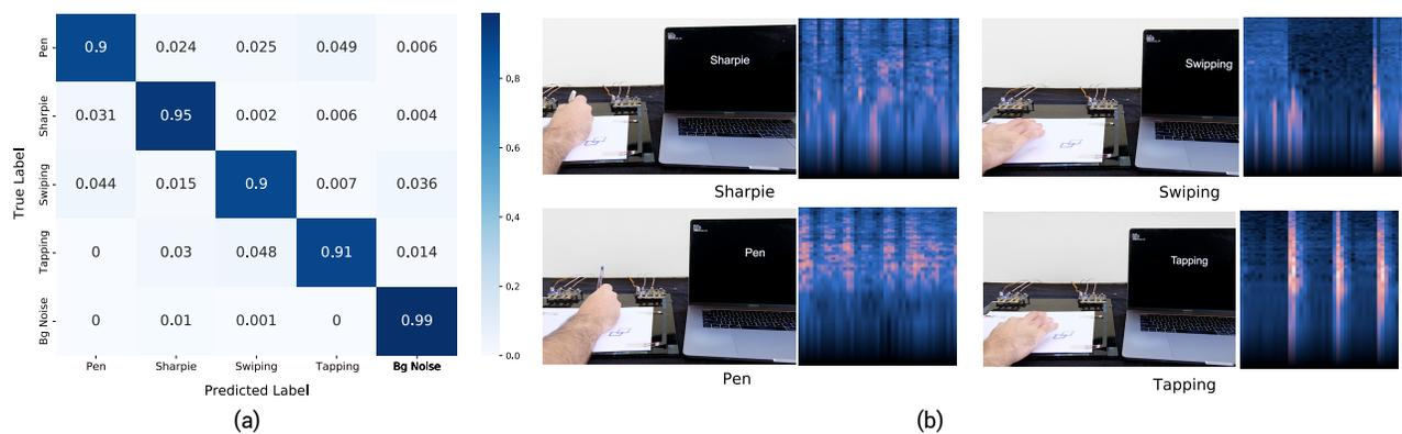
Figure 10. (a) 5x5 Confusion matrix evaluating the performance of our classification model predicting two instruments (pen and sharpie) and two hand gestures (tapping and swiping). (b) Images of interactions performed during evaluation and corresponding audio spectrograms.
