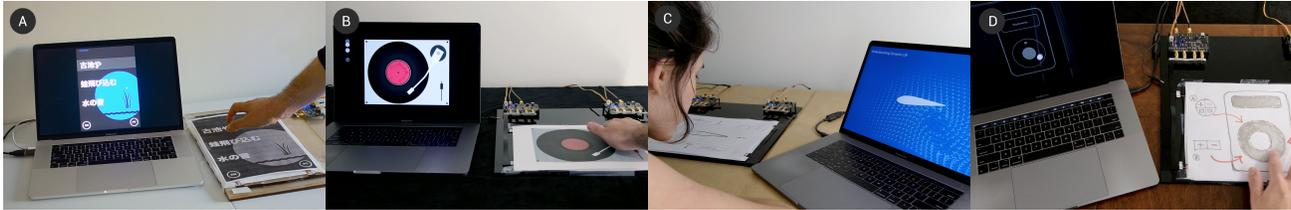
Figure 12. Example applications that demonstrate vibroacoustic sensing on paper. a) Touch to Translate Poster b) Paper Record Scratchin' c) BlowBased Airflow Simulation d) Digital Paper Prototyping.
