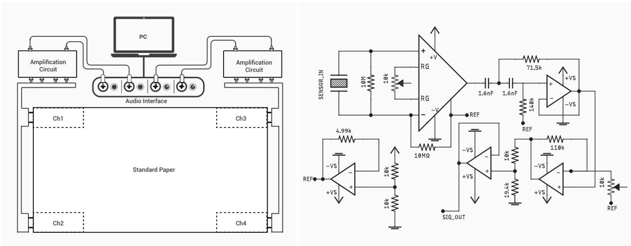
Figure 5. System setup of VibroAware. (Left) Each sensor is connected to an amplification circuit and an audio interface. The audio interface sends all channels to a computer to be sampled, then processed in real-time. (Right) The amplification circuit we designed for VibroAware. Each circuit has a 2-channel, 2-stage amplifier with a high pass filter and an analog output.
