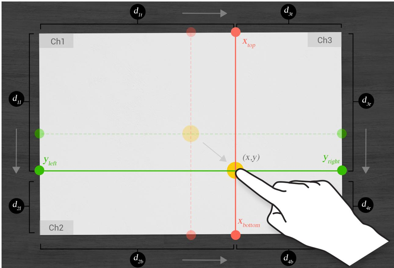
Figure 6. We use source localization to estimate the position of the contact point on a sheet of paper to enable paper-based interaction.
