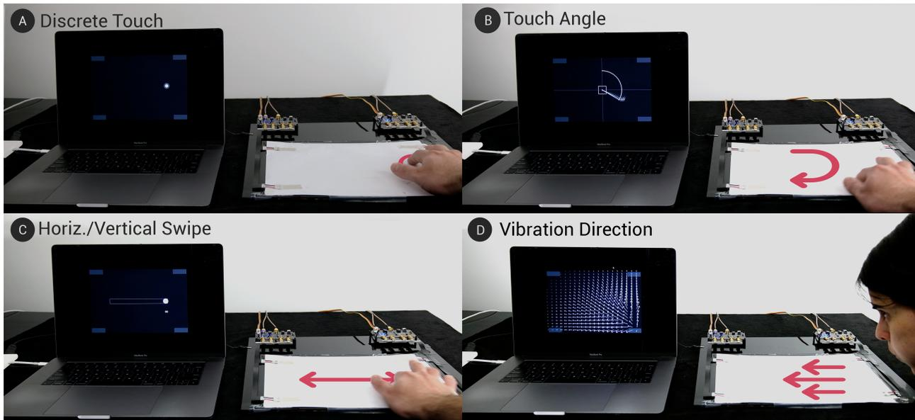
Figure 11. Image of interactions currently supported by our system. a) Discrete Touch b) Touch Angle c) Horizontal/Vertical Swipe d) Vibration Direction.
