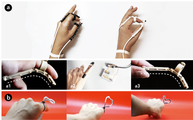
Figure 20: (a) Haptics-mediated sign language by record & playback of finger motions. (b) An OmniFiber-based ring morphing into an iconic heart shape as a tangible message.
