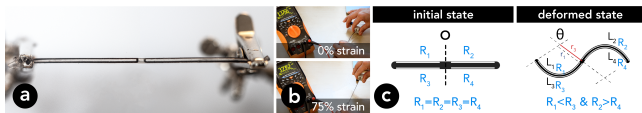
Figure 14: (a) 4-channel CB-based resistive strain sensor. (b) resistance values as 1,3MOhm at 0% and 3,2MOhm at 75% strain. (c) bending curvature principle diagram for an example double-bend deformation.
