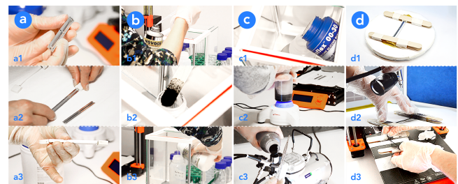
Figure 13: Step 2: Multi-step CB-based stretchable sensor fabrication. (a) Mask preparation: placing the tubing in the mask and clamping with screws. (b) CB powder-silicone solution preparation. (c) Mixing and pouring for spraying. (d) Applying airbrush at 15cm distance from the mask, and curing on 3D printer hot bed.
