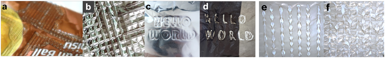
Figure 3: Embossing examples. Adjusting the Z-height of the extruder controls the depth of embossing pattern. (a) Hatch pattern engraved on a chip bag. (b) a checkered pattern, and (c) writing letters on the sealing layer of a retort food package, and (d) LDPE shopping bag. (e, f) Texture patterning by melting the material (HDPE) and dragging it. (e) By melting the starting point and dragging it to the next point, it can create the knitted-look-like pattern. (f) The same method was demonstrated in combination of X and Y direction.
