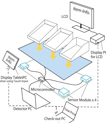
**Figure 3:** Base System Configuration.
