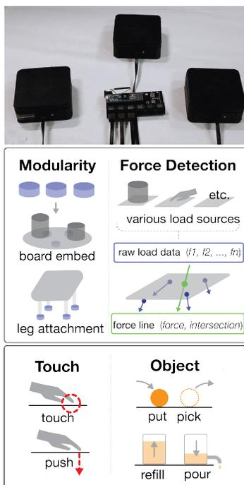
**Figure 2:** The SCALE tool kit which is shown in the top of the Figure, measures the intensity and direction of the applied force onto the weight sensing surface. Based on the force measurement, a designer can implement a variety of functionalities for touch detection and object status recognition.
