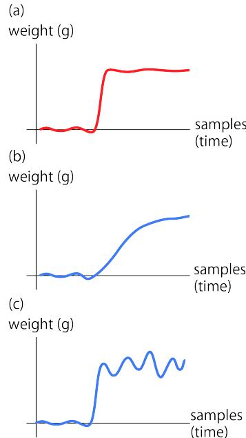
**Figure 5:** Object Recognition Sequence. The red line indicates the sequence of samples from the signal when picking-up an object. Whereas, the blue lines indicate the sequence of samples from the signal when touching an object or a shelf.
