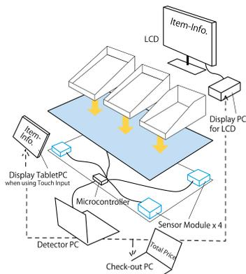
**Figure 3:** Base System Configuration.
