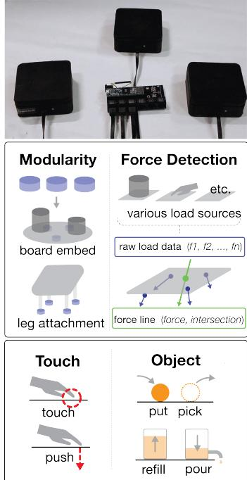
**Figure 2:** The SCALE tool kit which is shown in the top of the Figure, measures the intensity and direction of the applied force onto the weight sensing surface. Based on the force measurement, a designer can implement a variety of functionalities for touch detection and object status recognition.
