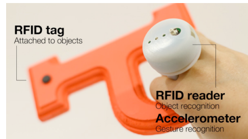
Figure 1: OnObject system involves RFID tags and a sensing device with RFID reader and accelerometer.
