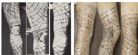
Figure 4. a) Iberall's depiction of the lines of non-extension, drawn on a mannequin b) re-creation of Iberall's lines on a full scale model with kevlar joints by MIT MVL
