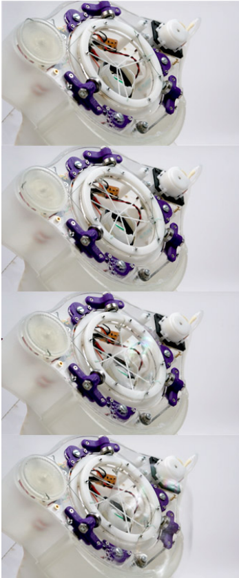
Figure 3: From closed position to open position of string iris mechanism (From top to bottom). As it open, the 3 lines of string form a triangle shape with bubble membrane.
