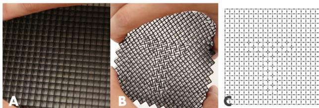
**Fig. 21.** Application: encoded display. Letter T. (A). before compression; (B). after compression; (C). hinge position.
