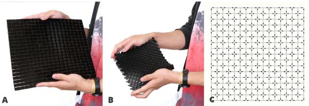
**Fig. 13.** A 15 by 15 identical unit KinetiX panel can be fabricated by simple propagation. The piece exhibits the known auxetic effect. (A). Printed piece; (B). After compression; (C). The hinge configuration.
