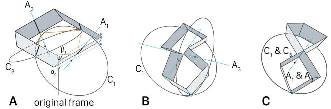
**Fig. 8.** (A). Initial transformation setup of out-of-plane rotation with corresponding labelling conventions; (B). Maximum transformation states under  $A_{wall-rot} = (\beta_m, -\beta_n, \beta_m, -\beta_n)$ ; (C). Maximum transformation state under  $A_{wall-rot} = (\beta_m, \beta_n, \beta_m, \beta_n)$ .
