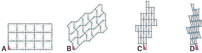
**Fig. 10.** Transformation of a  $3 \times 5$  grid-like tessellation with uncrossable linkage. (A). Initial setup of the frame; (B).  $45^\circ$  rotation; (C).  $90^\circ$  rotation; (D). some  $>90^\circ$  rotation in which frame parts start to intersect and produce physical collision in reality. The initial fixed triangle at the left-bottom corner is labeled in pink.
