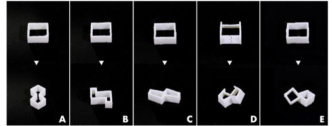
**Fig. 12.** Five fabricated unit of planar and spatial transformation. (A). the basic unit; (B). planar transformation of uniform scaling; (C). planar transformation of shearing; (D). spatial transformation of bending; (E). spatial transformation of twisting.
