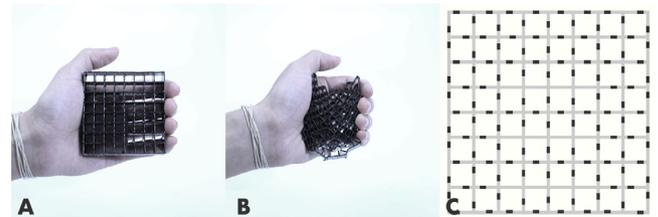
Fig. 14. An 8 by 8 gradient unit KinetiX panel. The hinges gradually shift their position from left to right. (A). Printed piece; (B). After compression; (C). The hinge configuration.
