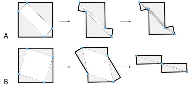
**Fig. 5.** A. Crossable linkage. Collision does not happen and the frame can continue to transform after the four-bar linkage coincide on a line. Hinges on the linkage will pass through the bars.  $P = (0.8, 0.2, 0.8, 0.2)$ ; B. Uncrossable linkage. Collision occurs and the frame cannot continue to transform when the four-bar linkage coincide on a line.  $P = (0.8, 0.8, 0.8, 0.8)$ .
