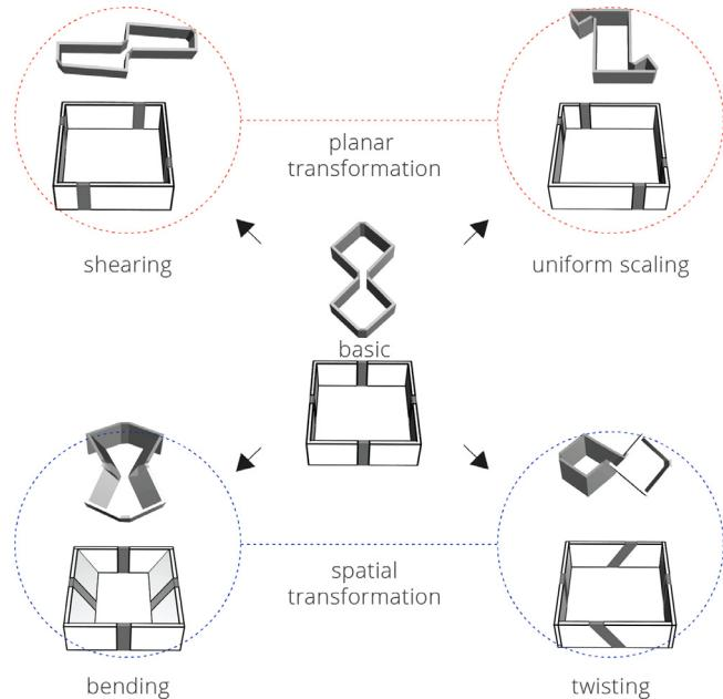
**Fig. 2.** The design parameters of KinetX. From the basic unit, a planar and spatial transformation can be created. Parametrically shifting the position of the hinge creates uniform scaling and shearing; rotating the hinge in or out-of-plane creates twisting and bending.
