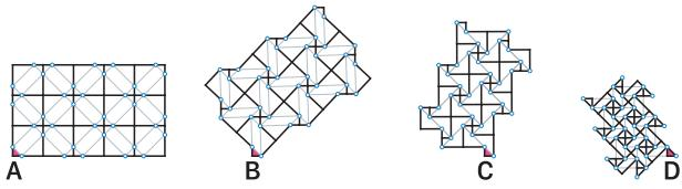
**Fig. 9.** Transformation of a  $3 \times 5$  grid-like tessellation with crossable linkage. (A). Initial setup of the frame; B.  $45^\circ$  rotation; C.  $90^\circ$  rotation; D.  $135^\circ$  rotation. The initial fixed triangle at the left-bottom corner is labeled in pink.
