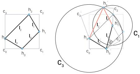
**Fig. 3.** Planar transformation deduced from the geometric relationship of intersecting circles.
