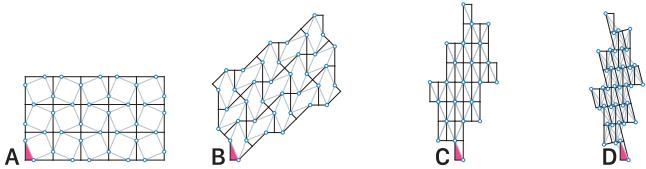
**Fig. 10.** Transformation of a  $3 \times 5$  grid-like tessellation with uncrossable linkage. (A). Initial setup of the frame; (B).  $45^\circ$  rotation; (C).  $90^\circ$  rotation; (D). some  $> 90^\circ$  rotation in which frame parts start to intersect and produce physical collision in reality. The initial fixed triangle at the left-bottom corner is labeled in pink.
