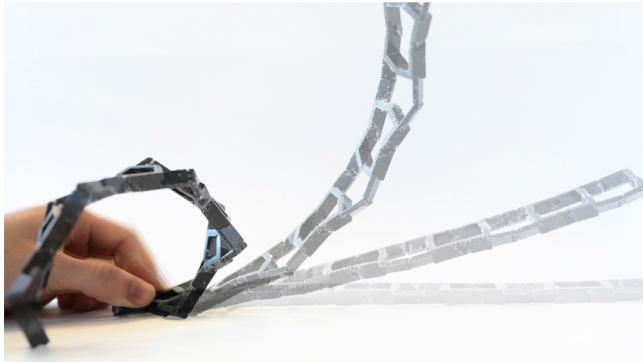
**Fig. 15.** A 1D tessellation of spatial transformation of bending and twisting. This tessellation creates a curling strip.
