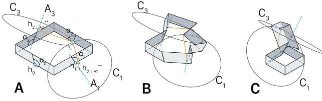
**Fig. 7.** (A). Initial transformation setup of hinge in-plane rotation with corresponding labelling conventions; (B). Unmatched state during the transformation; (C). special matched state with angle combination  $A_{in-plane} = (\frac{\pi}{2}, \alpha, \frac{\pi}{2}, \alpha)$ .
