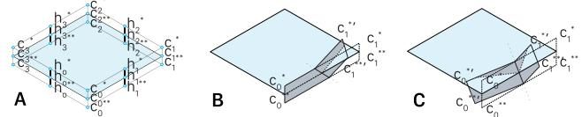
**Fig. 6.** (A) 3D hinged frame unit and labeling convention; (B) Hinge in-plane rotation; (C) Wall plane rotation.
