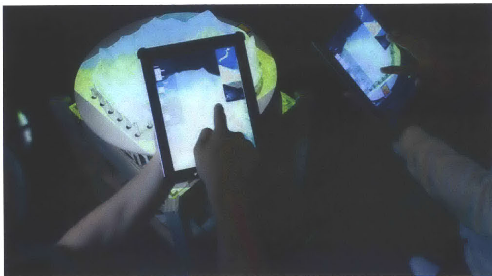
Figure 4-20: Multi-user geospatial data exploration. Hand-held tablets augment the shape display by adding layers of data, and extending the active workspace.
