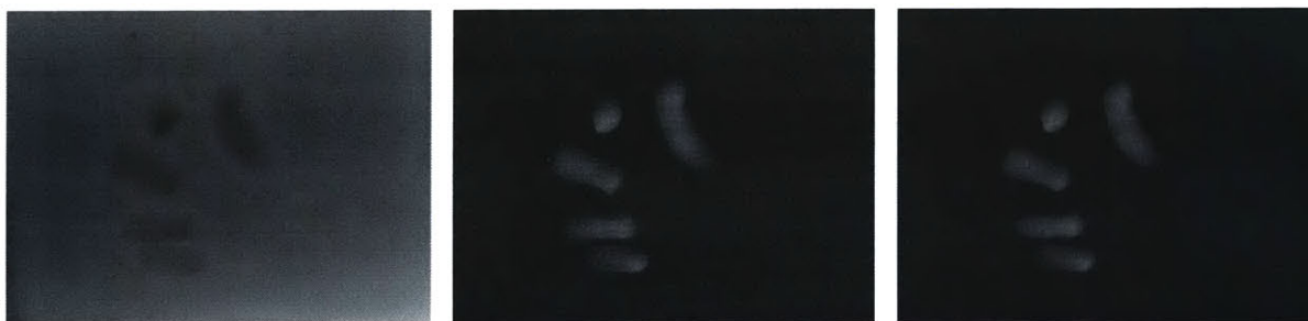
Figure 5-12: Tracking objects on deFORM. Left to right: Raw depth map of fingers pressed into gel; Background subtraction; Thresholded 2.5D image.
