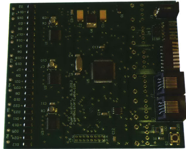
(b) The PCB Control Circuit for inFORM
