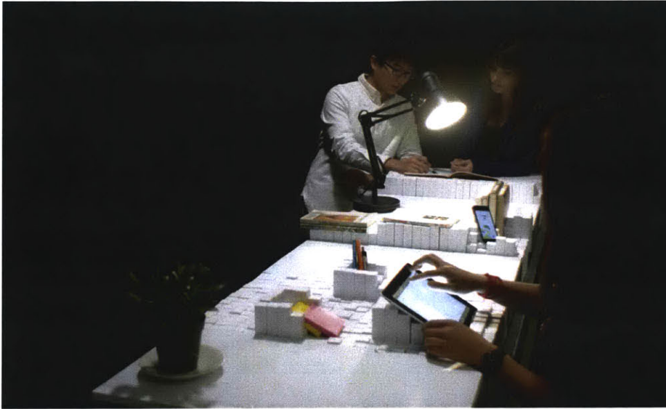
Figure 7-5: Transform, a shape-changing table, changes its shape to support different activities.
