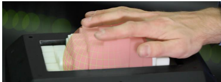
Figure 1: Mediate provides a mobile hand-sized shape-changing surface that renders coincident geometry of the virtual environment. Permission to make digital or hard copies of part or all of this work for personal or classroom use is granted without fee provided that copies are not made or distributed for profit or commercial advantage and that copies bear this notice and the full citation on the first page. Copyrights for third-party components of this work must be honored. For all other uses, contact the Owner/Author. CHI'18 Extended Abstracts, April 21–26, 2018, Montreal, QC, Canada © 2018 Copyright is held by the owner/author(s). ACM ISBN 978-1-4503-5621-3/18/04. https://doi.org/10.1145/3170427.3188472
