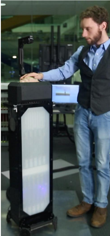
Figure 2: A user touches a virtual object on the pedestal-size mobile shape display.
