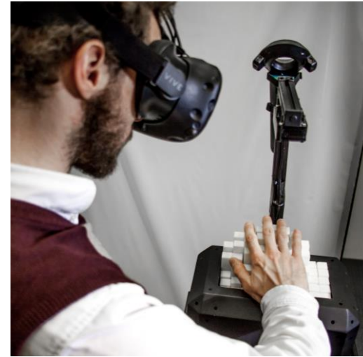
Figure 3: A user wearing an HMD interacting with a virtual object simultaneously rendered physically on Mediate
