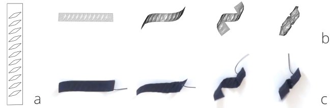
Figure 10. Given an encoded composite (a), our simulator is used to predict the inflated shape of the structure (b), which is in close agreement with the actual physical performance of the fabricated artifact (c).
