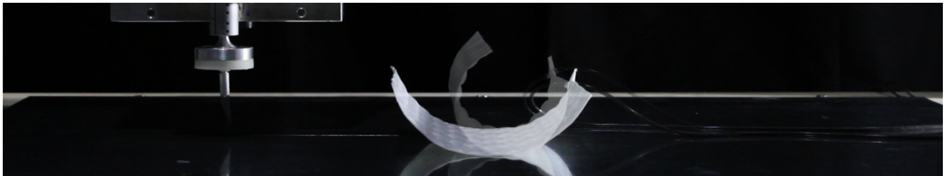
Figure 1. Heat-sealed rayon challis fabric changes its shape upon inflation
