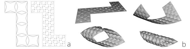
Figure 30. (a) The hinge design of the double layer structure. (b) Simulation of the lampshade folding.
