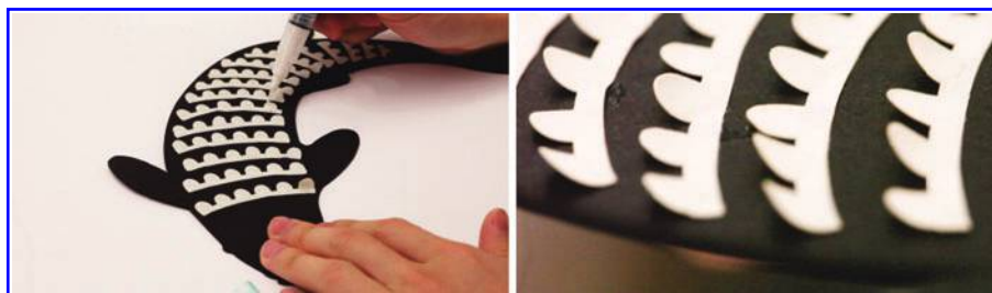
FIG. 5. Living paint. Spore solution as an active ink to actuate toy fish scales. Color images available online at www.liebertpub.com/3dp
