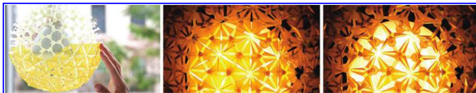
FIG. 17. Transformable lampshade. The flaps open up as the temperature rises, causing RH to drop. Color images available online at www.liebertpub.com/3dp
