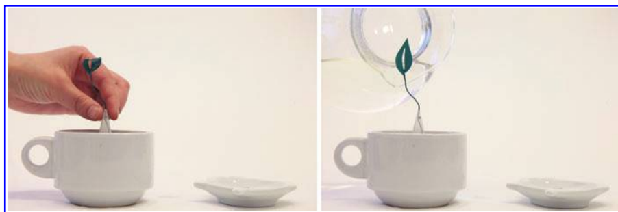
FIG. 16. A teabag with an artificial transformable leaf as an indicator. Color images available online at www.liebertpub.com/3dp
