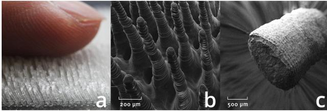
**Figure 10. (a) Printed hair structure with laser beam based SLA. (b) SEM photo of (a). (c) Oval shape of the laser beam.**
