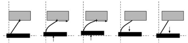
**Figure 18. One cycle of the stick-slip mechanism.**
