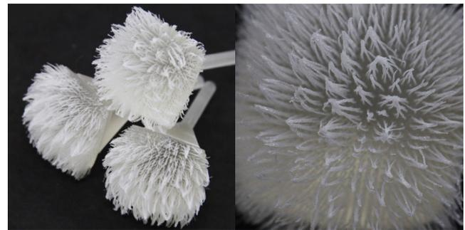
**Figure 9. Successful printed hair arrays on curved surfaces.**
