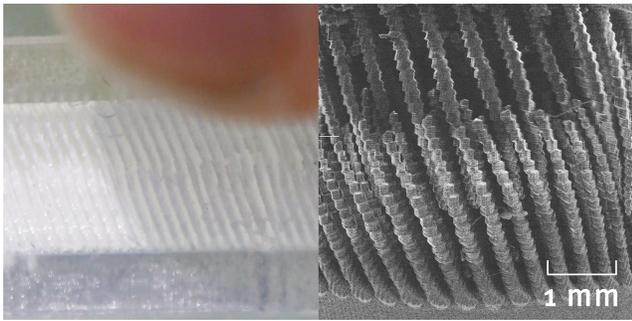
**Figure 16. Large amount of contact surface on the hair creates high friction.**
