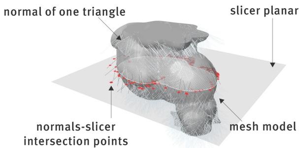
**Figure 8. Hair generating while slicing a mesh model.**
