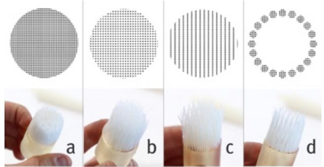
**Figure 13. Printed brushes with different density and style.**
