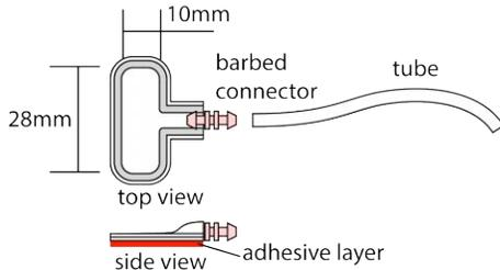
**Figure 4. Design of the square-shape sticker actuator.**
