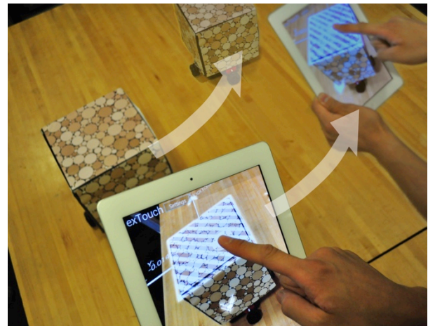
Figure 1. exTouch, User can simply touch and drag the target device through live video on the screen
