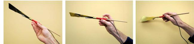
Figure 2: Holding the wand, pressing the record button to capture a sound sample, and scraping the wand against a wall to stimulate the sample.
