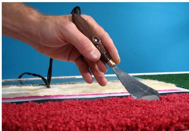
**Figure 1.** The Painting Knife tool is scraped against shag carpet, convolving a digital audio sample with the acoustics of the carpet's physical texture.
