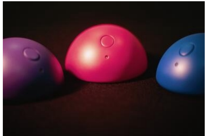
Figure 1: Three palm-sized curlybots (each with a large record/playback button and a small indicator light).
