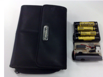
Figure 4. "Bumblebee" wallet: Concept sketch and photo of wallet with Bluetooth/vibration circuit removed.
