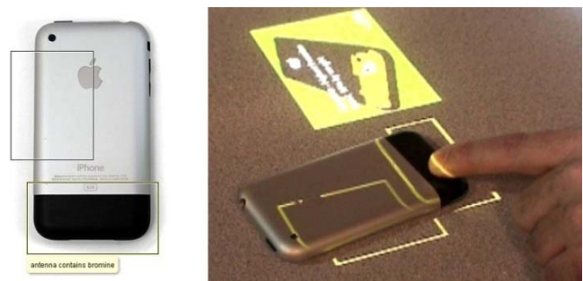
Figure 4. Product designers could place meta-data in specific parts of an object to assist in maintenance (simulation).
