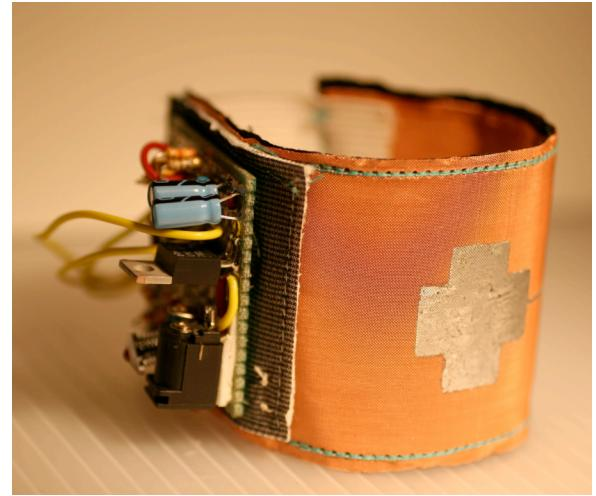
**Figure 1.** The electromagnetic field (EMF) detector bracelet.
