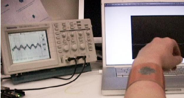
**Figure 3a.** The bracelet is located at 14 inches away from the display – the oscilloscope shows the front-end output.
