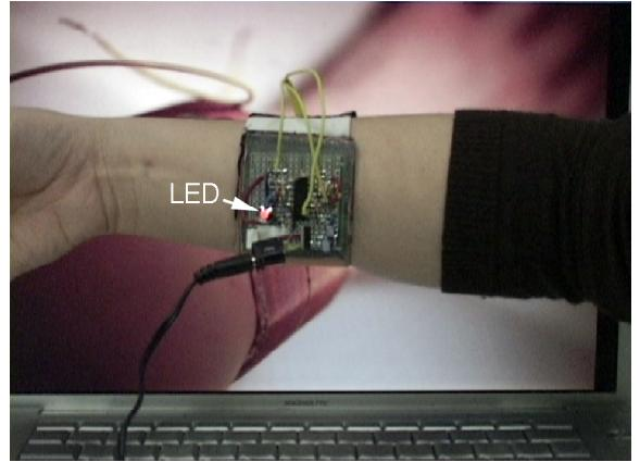
**Figure 4.** The battery-powered bracelet is at 1 inch away from the screen, where the feedback LED is fully illuminated.
