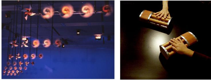
Super Cilia Skin is inspired by wind swept grass and explores how motion in an array of hair like actuators can be used as a textural communication device.
