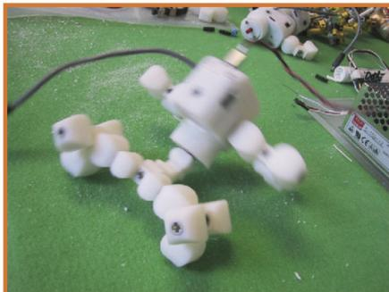
After the wooden prototypes, we modelled a plastic housing and printed plastic parts on an FDM 3D printer.
