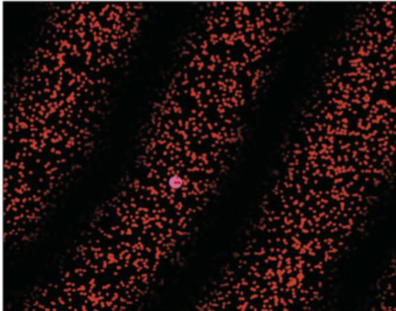
A plane-wave oscillator running on 10,000 simulated devices. The placement of source (yellow) and destination (magenta) markers in the devices' sensor field determines the wave's period and direction. In a kinetic mesh, the source and destination may be specified tangibly, e.g. by pressing buttons on nodes.
