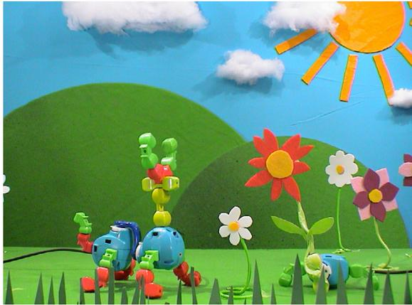
When a creation is in "playback" mode, joysticks adjust speed and amplitude of the motions. Continuously depressing a "reverse" button will cause a recorded motions to play backwards. (Reverse may cause a creature that walks forward to walk backwards.) Users of Robo can spontaneously control Topobo motions in real-time to create original sequences of movements.
