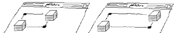
Figure 4. Two bricks can stretch the square. One brick acts like an anchor while the second brick is moved.
