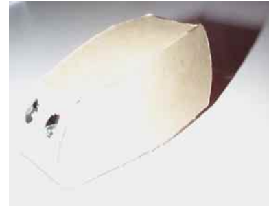
Figure 4.2 The hamster phicon (physical icon) is a small motorized representation, which vibrates when our real hamster is active.
