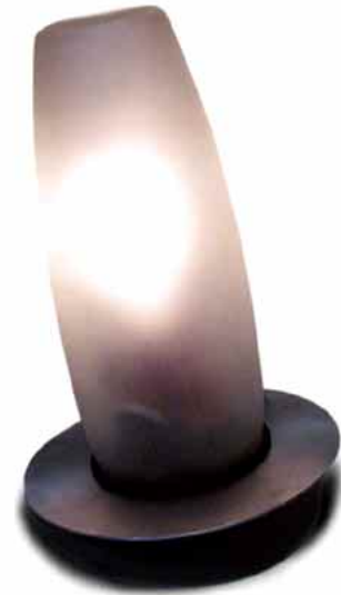
Figure 4.14 The wobble lamp is a table top lamp with the ability to physically move, or gesture.
