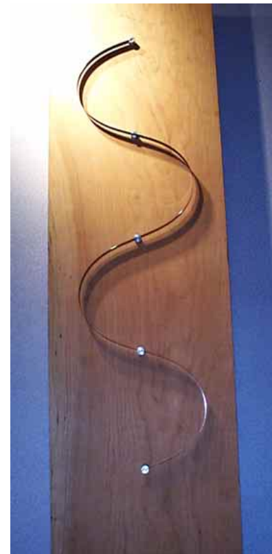
Figure 4.13 The spline is a flexible piece of springsteel with five rotary control points. It suggested intriguing ideas about more expressive and abstract physical displays.
