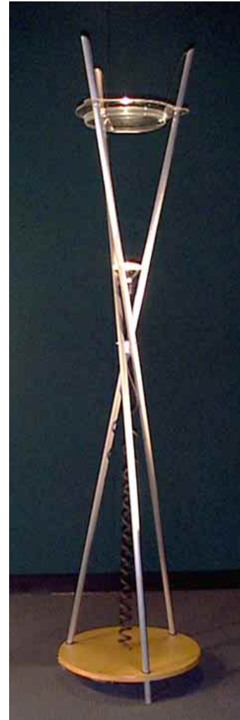
Figure 4.8 The water lamp is a free-standing floor lamp that can create subtle reflections of water ripples upon the ceiling based upon an information input.
