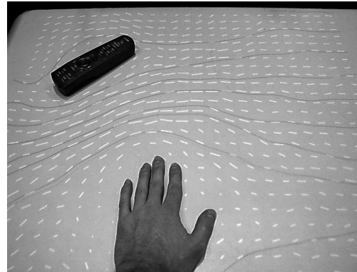
Fig 4: seep 's fluid diverted by physical obstacles
