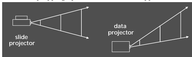
Fig 9: Normal v. 'anti-keystoned' projection
