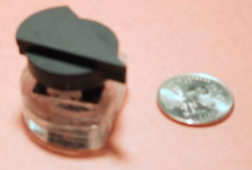
Figure 4: The top and bottom of a dial that plugs into a Sensetable puck.
