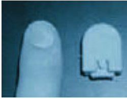
Figure 6: V1220 speaker actuator (a finger is included for scale)
