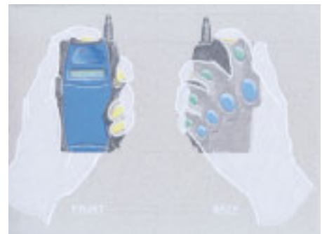
Figure 1: ComTouch Concept drawing showing a handheld sleeve that fits onto the back of a mobile phone
