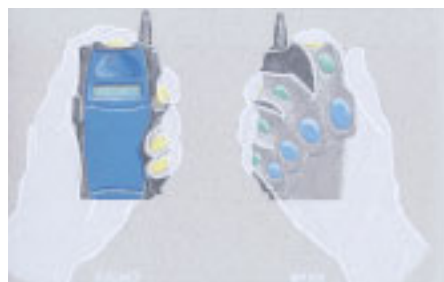
Figure 18: ComTouch concept drawing depicts the ergonomic grip.
