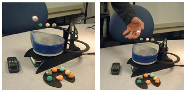
Fig. 1. At Jane’s end, the ball floats when a call comes in. She grabs the ball to answer the call.
