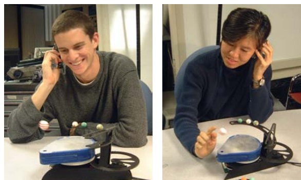
Fig. 3. In conversation: the ball floats up and down in correspondence to the remote person’s movement.
