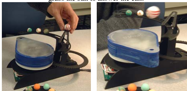
Fig. 2. The ball rolls down the ramp and an air stream levitates it.
