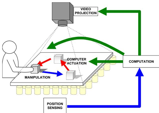
Figure 2: Traditional interactive workbench systems provide feedback through video projection alone. The Actuated Workbench adds an additional feedback loop using physical movement of the tracked objects.
