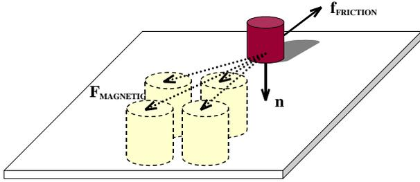
Figure 10: The electromagnets (lower left) exert forces on the puck (upper right).
