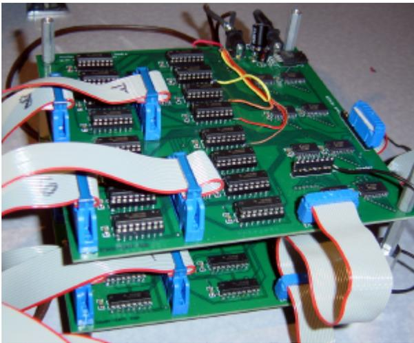
Figure 5: Custom-fabricated circuit board containing flip-flops and H-bridge transistor arrays.
