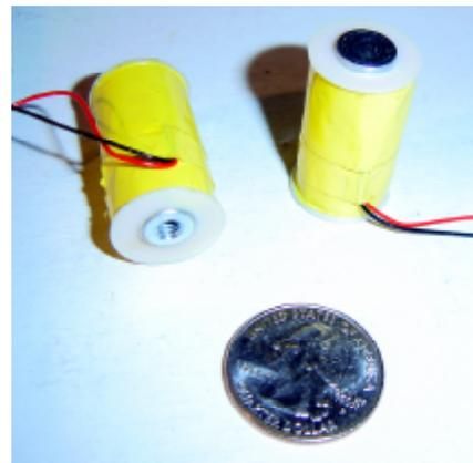
Figure 4: Custom-wound electromagnets produce broad, uncontained magnetic fields.
