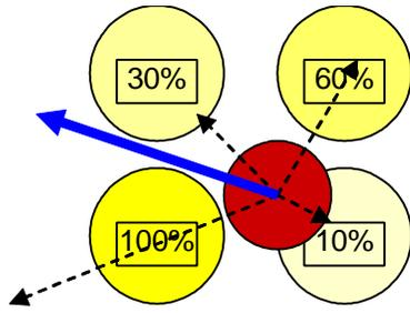
Figure 12: Four electromagnets with different duty cycles combine to produce a force with a new direction and magnitude.
