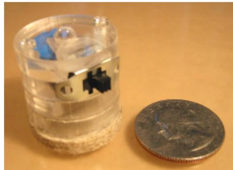
Figure 6: Our puck design includes a permanent magnet and an infrared LED for vision tracking.
