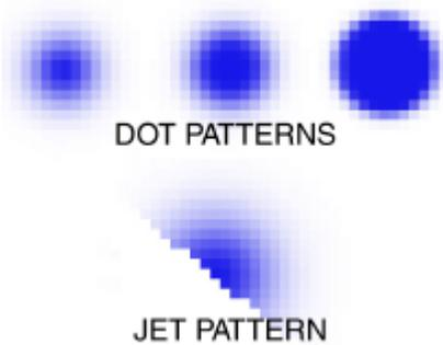
Figure 14: “Dot” and “Jet” equivalents in computer graphics (using a higher resolution grid than is present in our system). The three dots use different falloff metrics.
