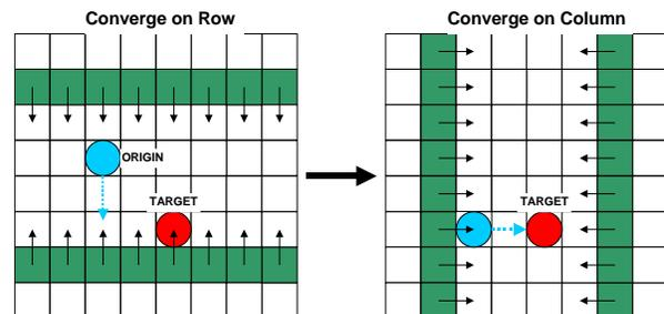
Figure 9: Sweeping to a desired point from an unknown origin.
