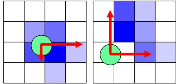
Figure 13: Anti-aliasing methods. The squares represent magnet cells, and intensity of each shaded square corresponds to the duty cycle of the magnet. The “dot” technique (left) results in slower travel than the “jet” technique (right).
