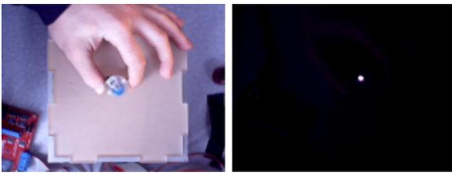
Figure 7: Overhead view of the Actuated Workbench from vision camera without IR filter (left) and with IR filter (right).
