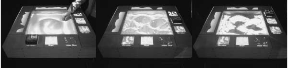
Figure 7 A number of different GIS analysis functions can be selected from the thumbnails around the worktable. From left to right: height, aspect, and shadow casting
