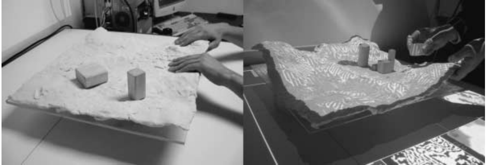
Figure 4 The tangible worktable comprises a landscape model, which is augmented by computer projections. In the Illuminating Clay case, any object from the user's environment can be used for including the user's own hands, pieces of paper, cardboard, foam, plastic or other objets trouvés
