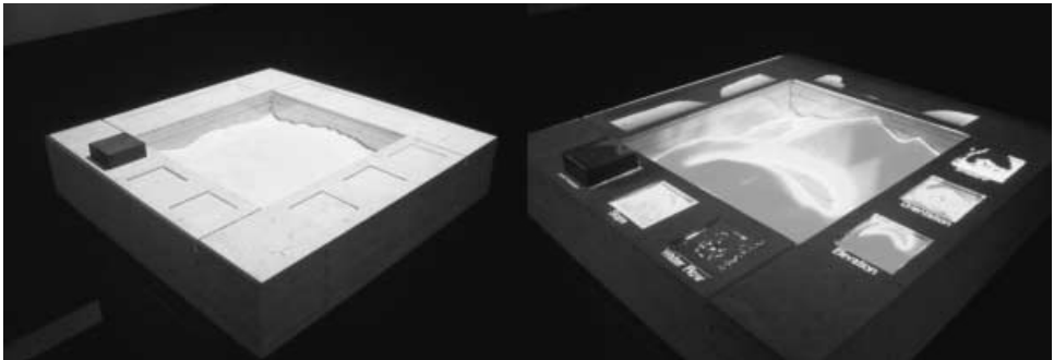
Figure 5 The tangible worktable in the SandScape system. The geometry of the landscape model is defined using glass beads
