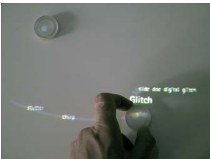
After a brief time delay, the floating menu moves back under the puck.
