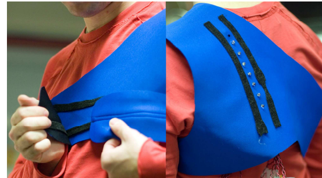
figure 3. The first actuators were held on to the body with a neoprene brace that ultimately proved too constraining and reminded one user of physical therapy.
