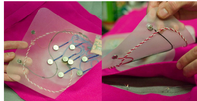
figure 4. In the most recent prototype, the flexible i/o haptic insert tucks into the felt scarf (left) and connects to central power through conductive steel snaps (right).
