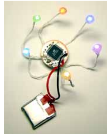
Figure 32: Six full-spectrum LEDs attached to a Glume nucleus.
