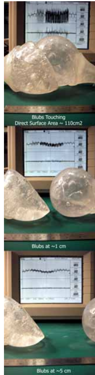
Figure 37: The amplitude of the capacitive coupling signal decreases rapidly as the bulbs are separated.
