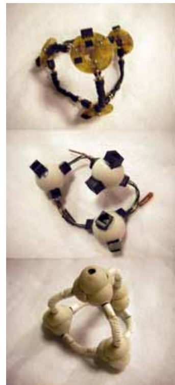
Figure 46: Evolution of the Senspectra toolkit. Top: First system with no strain sensors; Middle: Second system with resistive bend sensors on the joints; Bottom: Current system.
