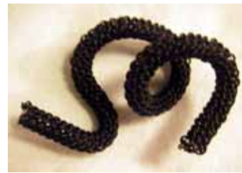
Figure 64: Plastic Joint prototype. This cable is embedded with titanium wire, a ductile metal that retains its shape when deformed.
