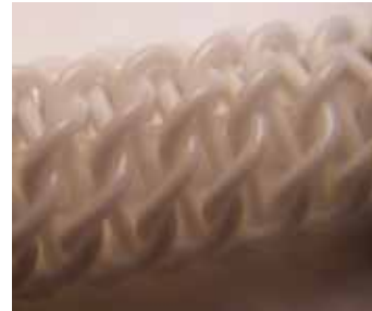
Figure 51: Braided wires around Senspectra's joints.
