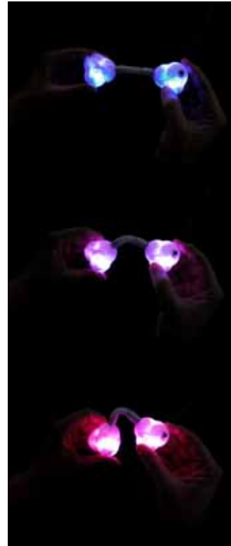
Figure 58: Simple Senspectra construction that changes color showing the mechanical stress between two nodes.
