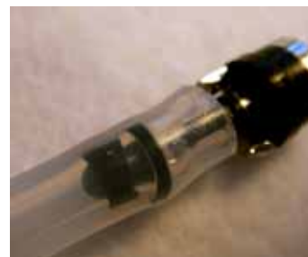
Figure 53: Phototransistor embedded in the silicone tubing that forms Senspectra's joints.
