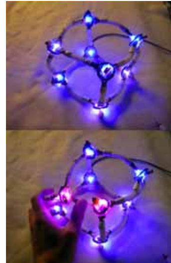
Figure 41: Senspectra structure reacting to the stress induced by a user's hand.
