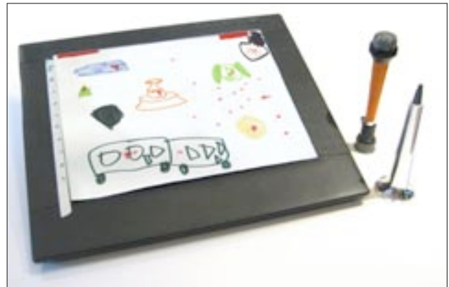
Figure 1. Children use Jabberstamp to create drawings with embedded audio recordings. Children use a special rubber stamp+microphone to record sound and a trumpet for playback. Paper and traditional art materials are used to create drawings.
