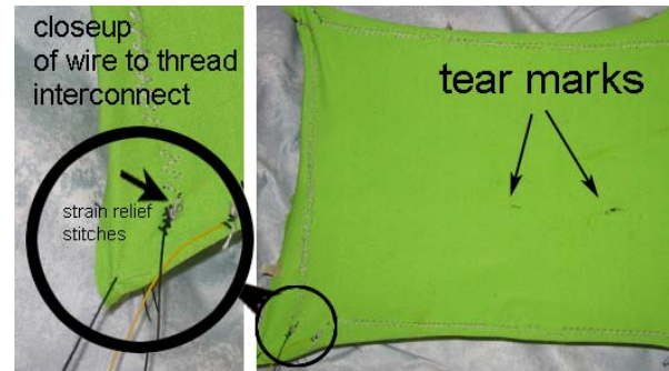
Figure 8. Holes and thread breakages on the fabric surface
